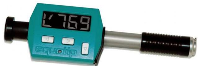
The Equotip Piccolo additionally allows for transfer of data to a PC.
