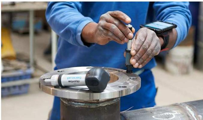
Equotip Live Leeb D is the world's first full internet of things portable wireless hardness testing solution. It brings real time data sharing, cloud backup and an intuitive user interface. The Live Leeb D is ideal for all those hard to access jobs.
