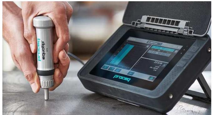
The Portable Rockwell hardness tester is ideal for thin and/or scratch sensitive and polished parts. Portable Rockwell gives excellent sensitivity through a small penetration of a few micrometres.
