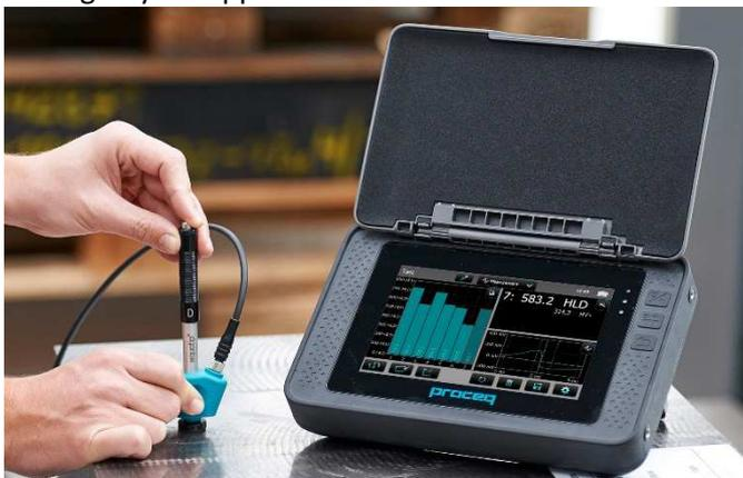
The Flexible UCI hardness tester is ideal for testing fine-grained material with and heat-treated surfaces. Testing heat affected zones and post weld heat treatment is a breeze with adjustable test loads from HV1 to HV5.
